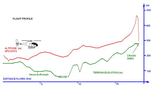
Fig. 9 – Flight profile (GPS data)
