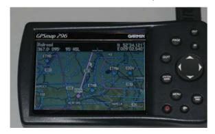
Positions derived from GPS signals are usually very accurate. However, this general accuracy can lead a pilot to believe that the instrument can do no wrong, which sadly is not the case. Since there is no integral monitoring system in most satellite navigation computers, there is no indication to the pilot that the information he thinks he is getting is incorrect. Only use GPS as a back-up to the normal primary means of navigation!
