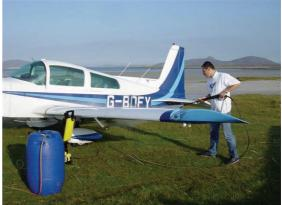
pressure washer, especially if you are attempting to wash off salt water a long way from the nearest source of fresh. However, by their very design, pressure washers are very likely to remove oil and grease from hinges and leave water behind. We therefore advise pilots not to use pressure washers, but if they do, have the aircraft re-lubricated immediately afterwards.
