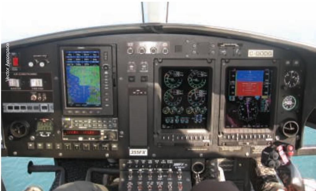
Vector Aerospace completed this panel upgrade in a Eurocopter AS355FX cockpit.
