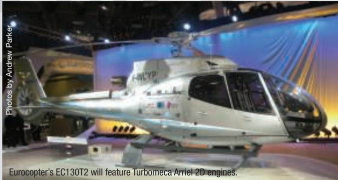
Eurocopter’s EC130T2 will feature Turbomeca Arriel 2D engines.
