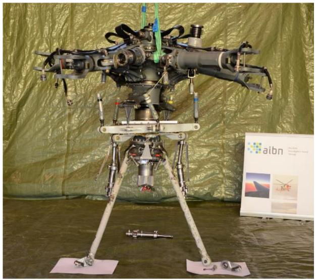
Figure 7: Main rotor head with rotor mast with aft suspension bars. Photo: AIBN
