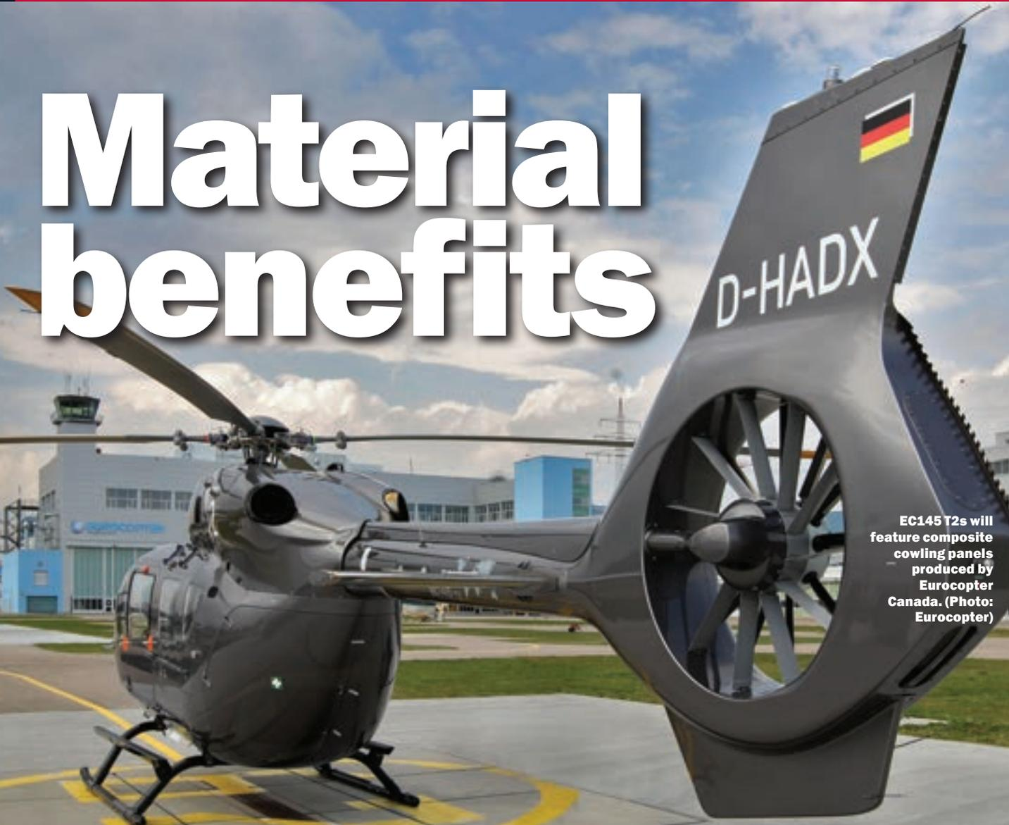
EC145 T2s will feature composite cowling panels produced by Eurocopter Canada. (Photo: Eurocopter)
