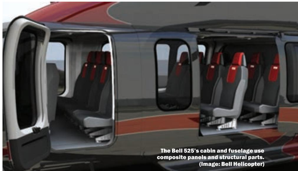
The Bell 525's cabin and fuselage use composite panels and structural parts. (Image: Bell Helicopter)
