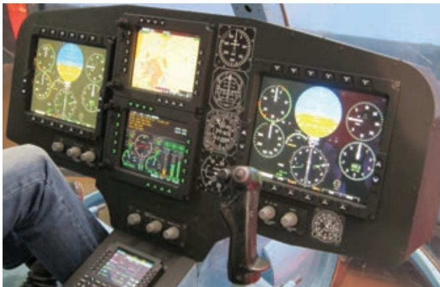
**This view of a simulator shows the Ka-226's typical cockpit layout, with flat-panel displays plus analogue backup instruments. (Photo: author)**
