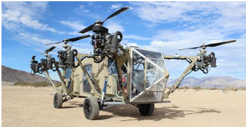
The AT Black Knight VTOL flying/driving pilot-optional technology demonstrator
