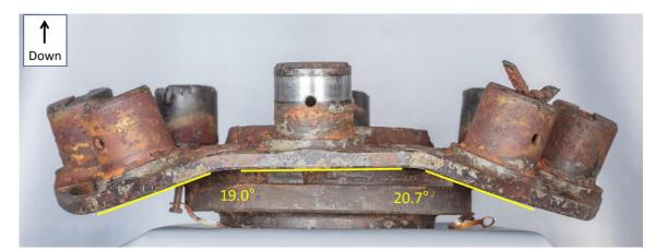
Figure 55. Deformation of carrier is symmetrical around the fractured planet gear. Photo: AIBN/QinetiQ
