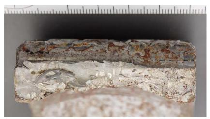
Figure 30: The cleaned through-thickness fracture surface. Macro marks (beach marks) are visible towards the upper edge of the gear (left hand side in photograph). Photo: AIBN/QinetiQ
