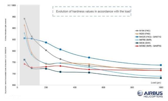
Figure 70: Hardness values vs. indentation load. From upper at the left hand side in the figure: FAG, FAG, FAG (QinetiQ), NTN-SNR, NTN-SNR, NTN-SNR (QinetiQ). Figure: Airbus Helicopters
