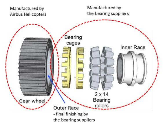
Figure 9: Second stage planet gear configuration. Source: Adapted from the AAIB / G-REDL report
