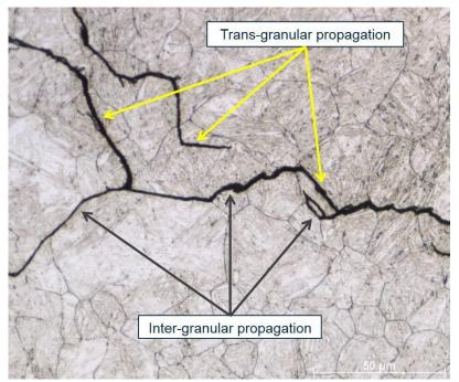
Figure 41: The subsurface crack propagation is both trans- and inter-granular. Roller direction to the left. Photo: AIBN/QinetiQ
