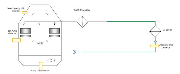
Figure 10: Chip detection system overview. Source: Airbus Helicopters
