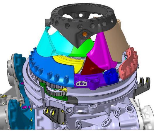
Figure 58: Illustration of how the retrieved fragments of the conical housing are pieced together in order to look for break-up sequence/mechanism. Illustration: Airbus Helicopters
