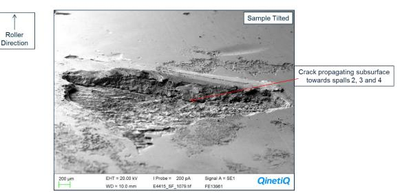
Figure 36: Spall one looking in the direction of spall two (in roller direction). A crack continuing under the surface is observed. Photo: AIBN/QinetiQ
