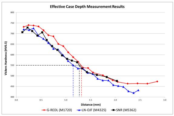
Figure 69: Outer race hardness values, comparison between a NTN-SNR gear, LN-OJF and G-REDL Figure: AIBN/QinetiQ
