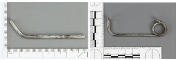
Figure 62: Two segments of safety pins found near the rotor mast. Metallurgical examination proved these to be from two different pins. Photo: AIBN/QinetiQ
