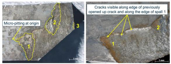
Figure 50: Fracture surface showing the extent of spalls 1 and 2. Photo AIBN/QinetiQ
