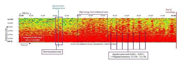
Figure 17: Spectrum analysis from the CAM audio file showing 1.3 seconds believed to be the beginning of the MGB break-up. Source: BEA
