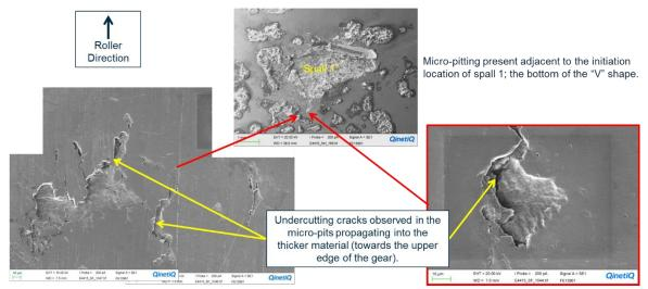
Figure 49: The micro-pits in the area in front of spall 1 Photo: AIBN/QinetiQ
