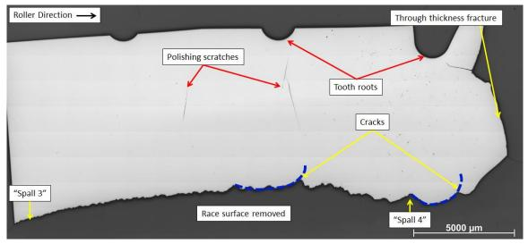
Figure 43: Sample FE13961 (see Figure 40). The micro-section is further polished to 15 mm from upper edge with the raceway removed. The micro-section shows deviations towards the gear teeth. Photo: AIBN/QinetiQ
