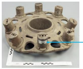
Figure 52: The second stage planet carrier found in February 2017 shown after cleaning. The inner race of the fractured second stage planet gear has been removed from stub shaft number 3 in front. Photo: AIBN/QinetiQ
