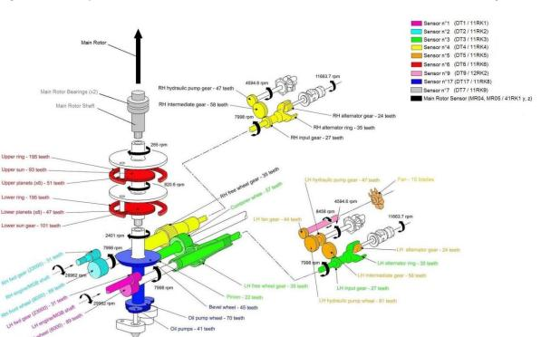
Figure 18: Drive train of the EC 225 LP M'ARMS<sup>™</sup> (MGB). Source: Airbus Helicopters
