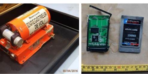
Figure 15: CVFDR from LN-OJF as received at Figure 16: HUMS PCMCIA card. the AAIB. Photo: AIBN
