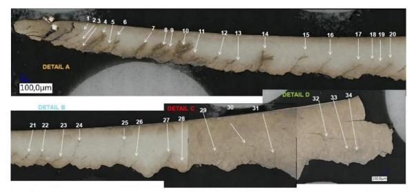
Figure 45: Polished section at the 14 mm line of the removed area (cap/calotte) between spall 3 and 4. Photo: Airbus Helicopters
