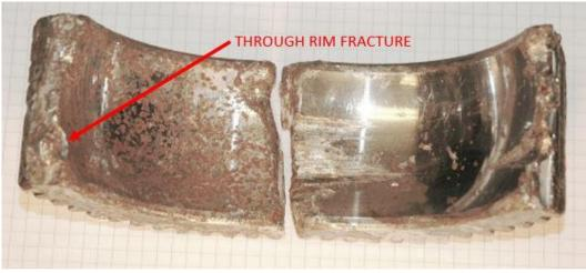
Figure 27: The two segments of the fractured second stage planet gear (serial number M4325). The fatigue fracture through the rim (through-thickness fracture) started in the outer upper race of the planet gear wheel where the red arrow is pointing (spall 4). Photo: AIBN/NDL
