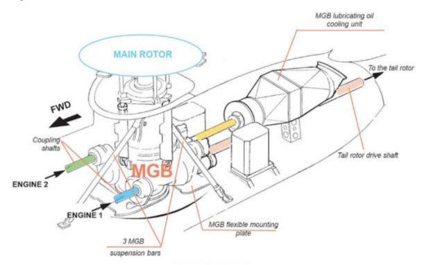
Figure 4: Transmission layout schematic diagram. Source: Airbus Helicopters
