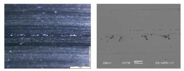
Figure 72: Micro-pitting within the dark line on gear M5769. Photo: Airbus Helicopters
