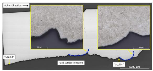
Figure 44: Sample FE13961 (see Figure 40). The micro-section shows a close up of deviations towards the gear teeth. Photo: AIBN/QinetiQ
