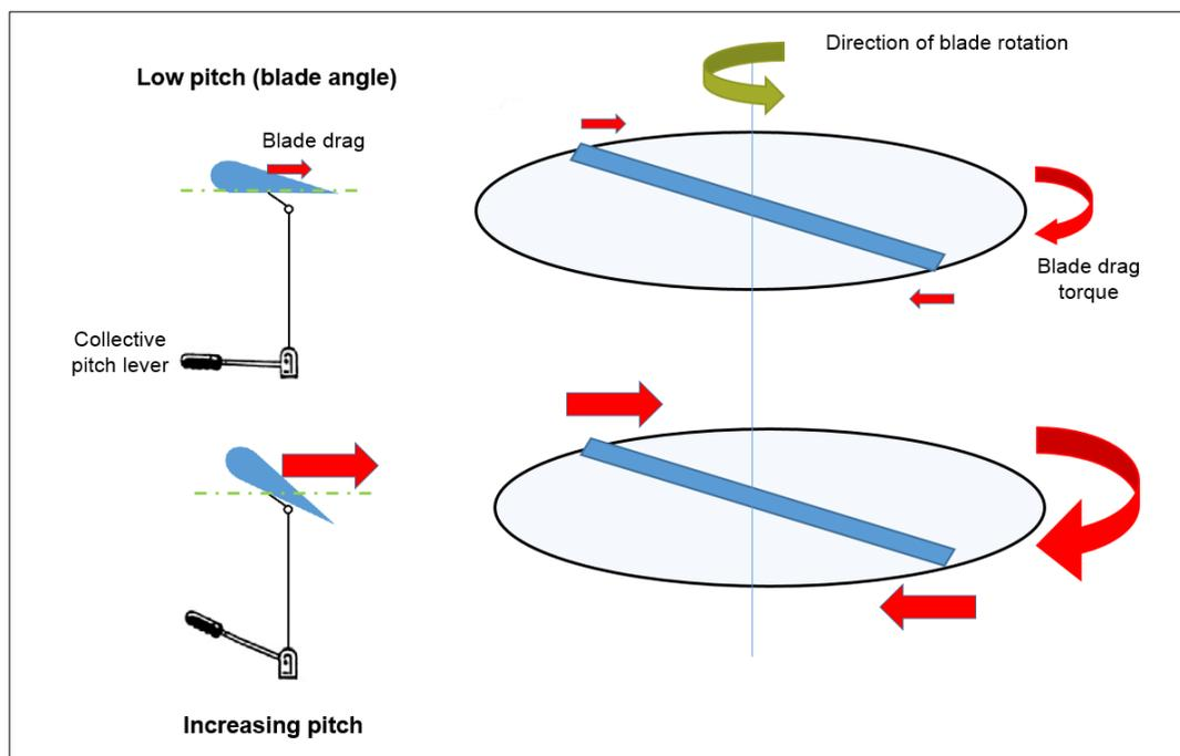
Figure 18: Sketch showing the increase in drag torque when pulling the collective lever
