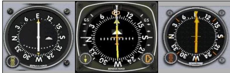
Aircraft heading and navigation instruments
